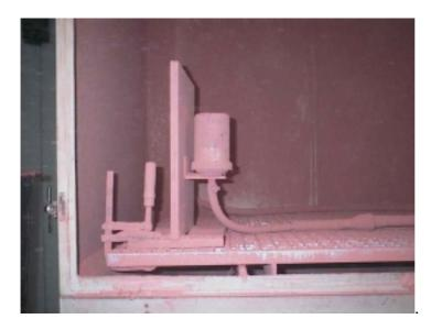
After the test the sample was inspected for the ingress of dust :
