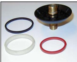
The white, red, and black plastic timing rings are used to set the frequency of ejection cycles of the MEMOLUB<sup>®</sup> HPS. They are inserted into the black plastic ring-holder either individually or in combination to obtain the desired frequency of output cycles.
