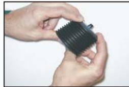
3. Carefully squeeze air out of the cartridge until grease begins to emerge from the outlet.
