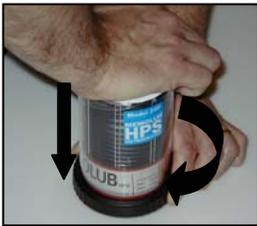
To close, use the same technique. Pressing down on the housing, hold the locking ring by its ribbed surface and turn it clockwise until it clicks into the locked position. Ensure that the locking ring locks by holding the ring on its smooth surfaces and turning clockwise. If the housing is correctly locked into place, it will not be possible to open it while holding the locking ring on its smooth surfaces.
