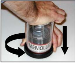
To open, place the lubricator upright on a flat surface. With one hand on top of the transparent housing, press firmly. With the other hand, hold the ribbed surface of the locking ring and turn it counter-clockwise. Remove the locking ring and the transparent housing.
