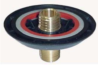
The MEMO regulates the rate of grease output of the MEMOLUB<sup>®</sup> HPS. It consists of a brass adapter, a black plastic timing-ring holder, and three plastic timing rings (one white, one red, and one black). The MEMO is permanently fitted onto the bearing or other component, and all MEMOLUB<sup>®</sup> HPS lubricators of any size will recognize its program setting.
