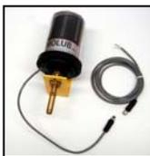
The EPC (External Power Control) version of the MEMOLUB<sup>®</sup> HPS is ideal for avoiding over-lubrication in applications where machinery is used infrequently or intermittently. The MEMOLUB<sup>®</sup> EPC operates under its own battery power but the lubricator is turned on and off externally. A 12" lead-wire extending from the base of the lubricator is connected to a relay. This relay is opened and closed in concert with the on-off switch of the machine on which it is being used.
