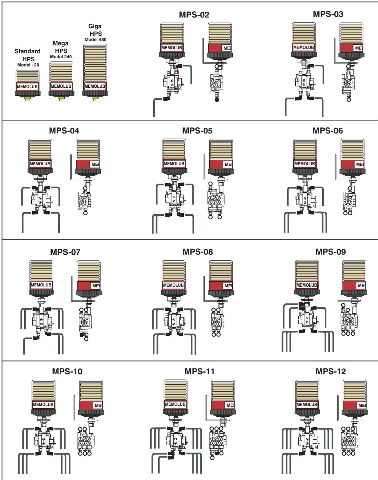
**Multi-Point Lubrication Distribution Block Set-Up**
