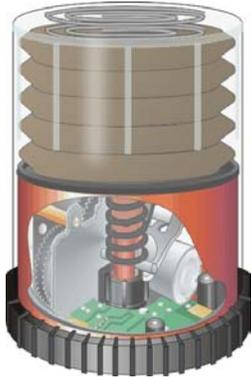
The lubricator body consists of a red motor housing, a transparent dome, a spring, a compression plate, a black rubber seal, and a black locking ring. The red motor housing contains all of the electro-mechanical parts of the MEMOLUB® HPS. The black rubber seal covers the battery compartment. Because of the configuration of its grease cartridge, the Model 480 lubricator does not require this black seal.
