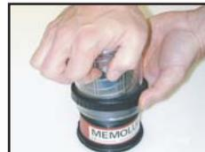
5. Place the clear housing assembly over the lubricant cartridge and red housing.
