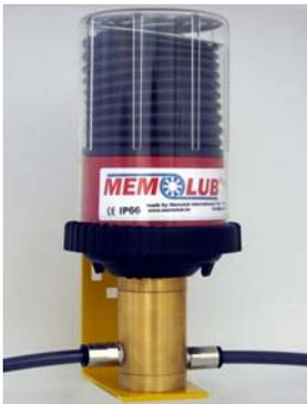
The Splitter-MEMO divides the volume of lubricant at each ejection cycle of the MEMOLUB<sup>®</sup> HPS. It is specially designed for the economical lubrication of two-bearing shaft systems such as electric motors, pumps, and fans. It transforms the MEMOLUB<sup>®</sup> HPS into a two-outlet system.
