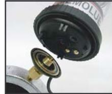
3. Screw the MEMOLUB<sup>®</sup> 24VDC-PLC on the Power-Through Memo fitting.
